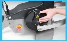
Release tension of the guide-string by using the free-coupling.
