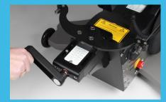
Turn the handle into position according to the stop-screw. Tension increases by turning the handle to the right.
